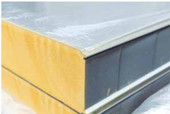
Two-component, solvent-free **PU adhesives** consist of a polyol (component A) and a hardener (component B). For their use, these components must be mixed in a certain proportion, which will depend on the product in question.
